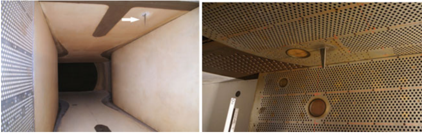
(a) T-128 wind tunnel nozzle and rake installed on its upper wall (b) Rake installed on the perforated upper wall of test section
