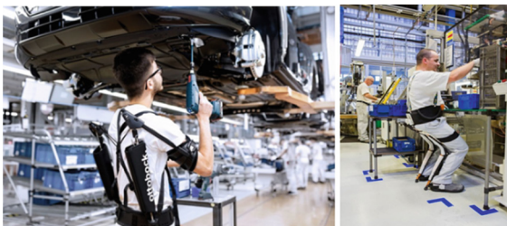
Fig. 1. Wearable upper body exoskeleton suitable for overhead work (left) and for lower body suitable for work in various working positions (right)
