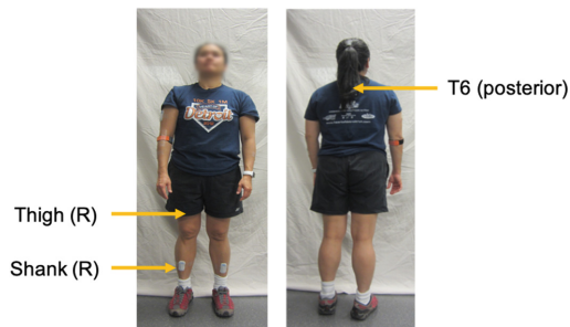
Fig. 1. Images depicting the three anatomical locations for inertial sensors attachment, namely, at T6, thigh (right), and shank (right).
