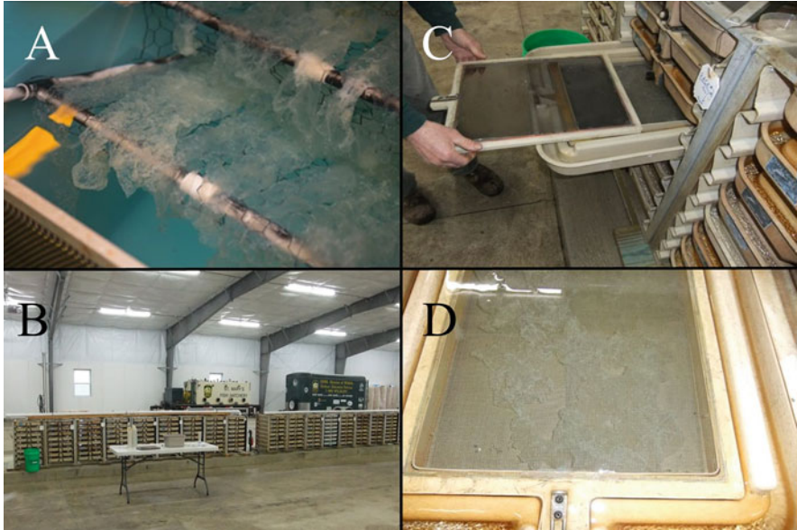
Fig. 2 Comparison of the Tank Racks and Heath Trays used by St. Marys SFH for egg incubation. (a) Tank Racks are made with 0.5-inch PVC pipe and wire mesh and are set at a 60° angle with egg ribbons anchored at the top, set between the wire mesh to remain submerged (Photo credit: Mark Pummell). (b) Heath Tray stacks at the St. Marys SFH (Photo credit: David A. Culver). (c) Each Heath Tray unit consists of eight trays with screens covering the egg ribbons to prevent loss as water flows via gravity from the top tray to the bottom tray (Photo credit: David A. Culver). (d) Egg ribbons incubating inside a single Heath Tray (Photo credit: David A. Culver)
