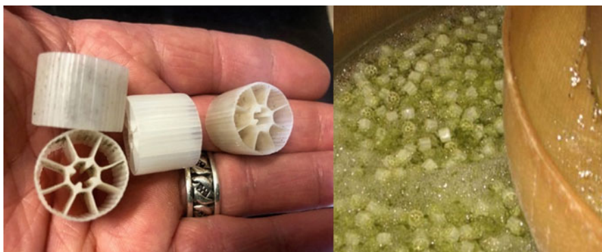
Fig. 6 MB3 media (left) was used as a surface for nitrifying bacteria in the MBBR (right)
