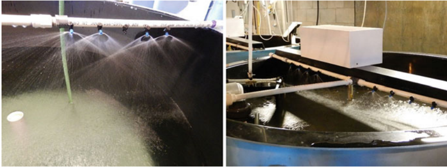
Fig. 11 Surface spray on the radial arm of the standard tank with bucket screen removed (left), spray bar spanning a self-cleaning tank (right)
