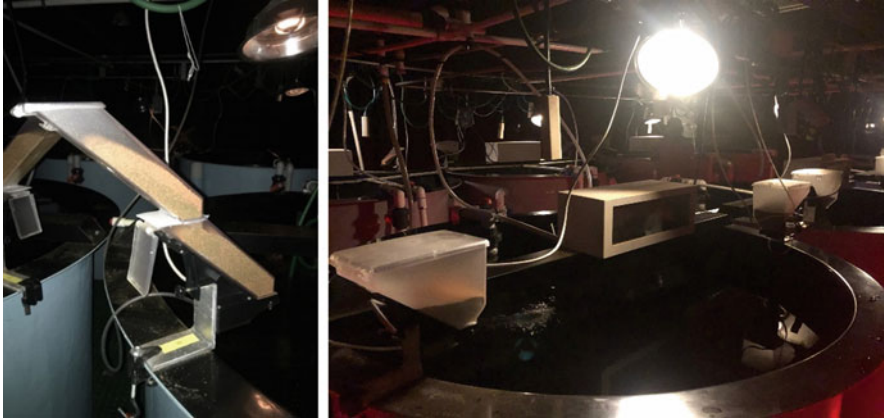
Fig. 17 Position of mounted HFS feeders on tanks: (left) a custom design modification of joining two 250-g hoppers together for increased capacity, (right) photo of 1-kg-size hoppers
