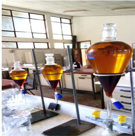
Fig. 4. Glycerol Separation from methyl ester
