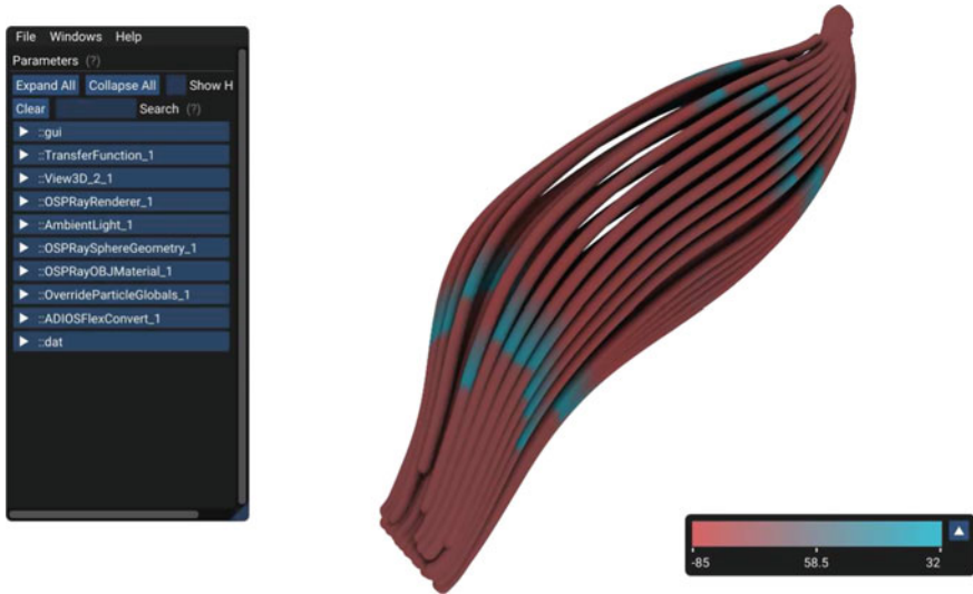
Fig. 9 In situ visualization of muscle fibers in the proof-of-concept in situ test case. In this case, we use a built-in opendihu simulation scenario with multiple muscle fibers and the mapped electric transmembrane potential, V_m . The simulation is connected to the visualization framework MegaMol
