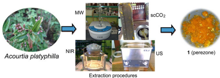
Fig. 8 Extraction of perezone (1) comparing NIR, MW, US, and scCO 2 . Adapted from Ref. [99]
