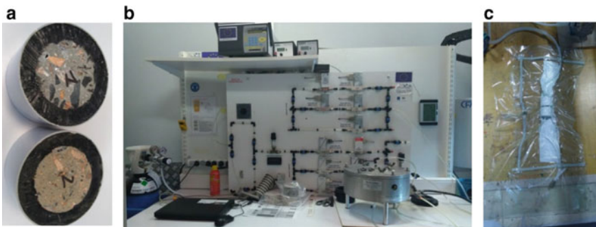
Fig. 3 a Samples P-01 and P-02 prepared for the air permeability test; b flowmeter massique equipment; c system used for the apparent porosity test
