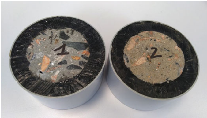
Fig. 6 Samples P-01 and P-02 prepared for the gas permeability test
