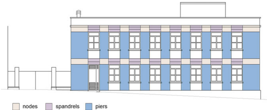
Fig. 18 Nodes, spandrels and piers of the east wall of the building
