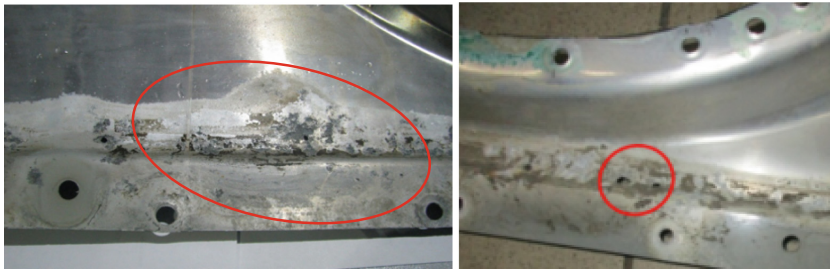
Fig. 2. Sill panel internal corrosion
