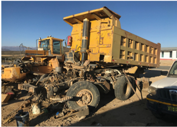
Fig. 2. Inoperative equipment used as a source of spare parts
