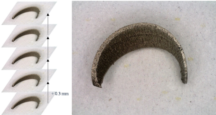
Fig. 1. Focus sequence (left) with an increasing z of 0.3 mm and the resulting all-in-focus image (right) from EDoF
