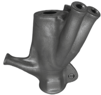
Fig. 7. Printed optimized node
