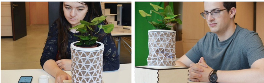
Fig. 4. Test set up (left: stretched position - right: slightly corrugated position)
