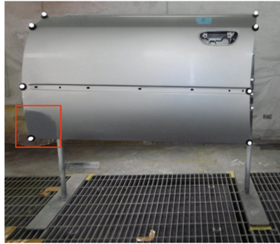
Fig. 1. Photograph of a door with a damaged part at the lower left 100 mm.
