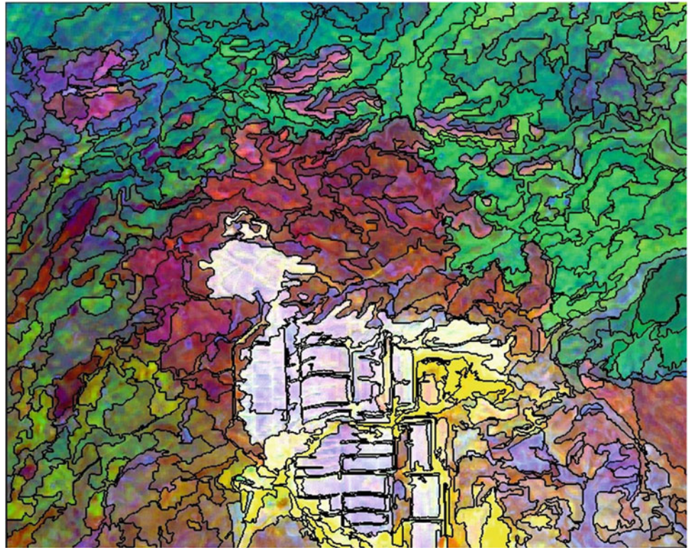
Fig. 6 The MRS result on the background colour composite image of the first three MNF bands
