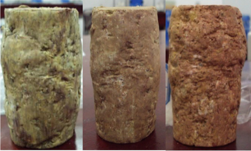
Fig. 9. The failure mode of granite residual soil samples after the CU tests
