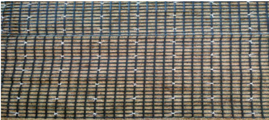
Fig. 1 Hybrid geosynthetic using coir geotextile and polyester geogrid
