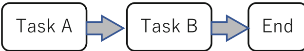
Fig. 6. Elimination of ‘and-join’ is the best way to suppress omission error. By transforming paralleled workflows to one stream in a fixed order, it will be easy to remember and to manage than and-join for human workers.
