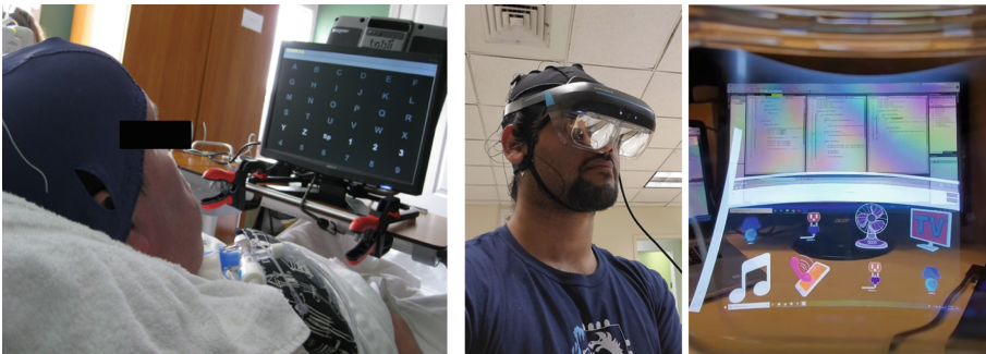
Fig. 1. Our traditional BCI set-up with a computer monitor screen (left). Augmented Reality glasses worn with an EEG cap (center). Augmented Reality display (right)
