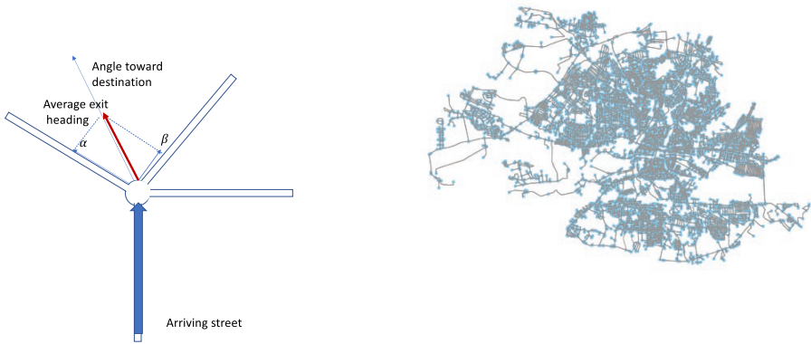
Fig. 3. Left: Illustration of steps of the randomized geo-routing algorithm. The traveller enters the intersection via the large blue arrow. Right: the map of Kaliningrad. (Color figure online)
