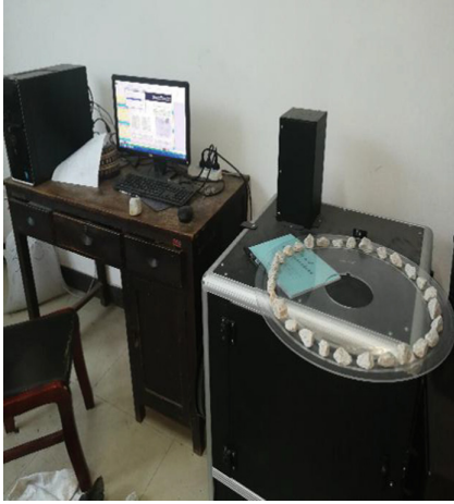
Fig. 2. Second-generation of aggregate imaging measurement system (AIMS)
