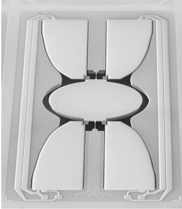
Fig. 18.27 PZT actuated quasi-static mirror. SEM picture
