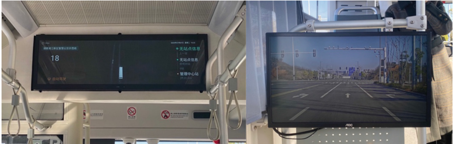
Fig. 1. Map and basic information display screen (left), Real-time return video display screen (right).
