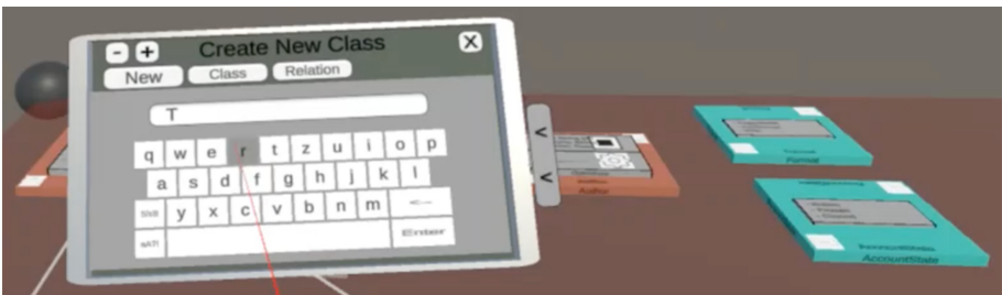
Fig. 8. VR-UML create class modeling support with virtual tablet and virtual keyboard.
