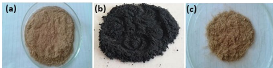
Fig. 1 a Photograph of raw Rice Straw. b Calcined \text{CoFe}_2\text{O}_4 nanoparticles and c prepared Rice Straw- \text{CoFe}_2\text{O}_4 nanocomposites
