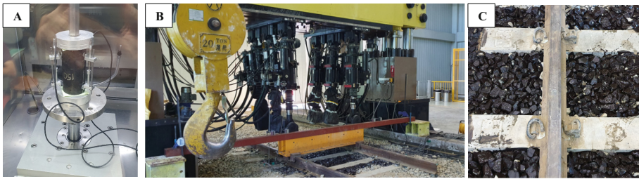
Fig. 1. Dynamic modulus test (a), full-scale testbed application (b), and CAM section (c).
