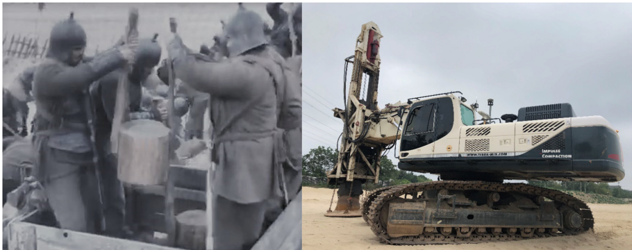
Fig. 1. Compacting in the past, stomping (left), and now, impulse compactor (right)
