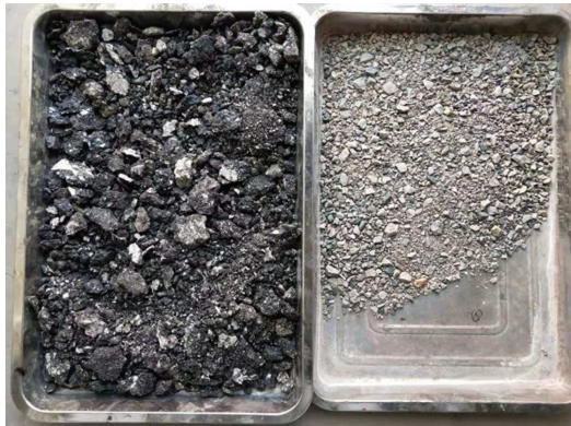
Fig. 1. Comparison of RAP material before and after asphalt analyzer
