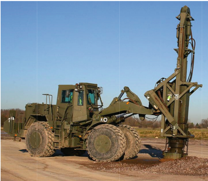
Fig. 3. British Ministry of Defence DV104 compactor or rapid runway compactor
