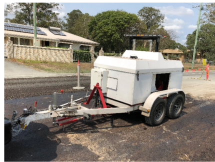
Fig. 7. Falling weight deflectometer (FWD) test
