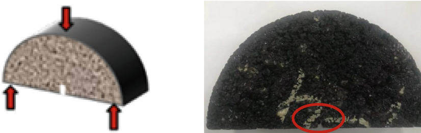
Fig. 3. SCB test principle diagram and the SCB specimen after cutting
