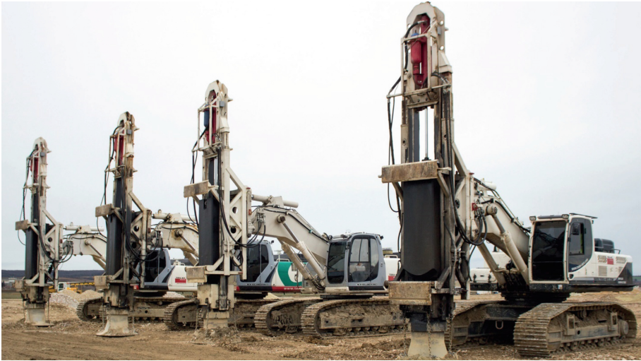
Fig. 18. Four impulse compactors ready for use in Nitra, Slovakia
