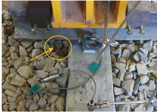
Fig. 8. The holes and separating of underlined ballast particles.
