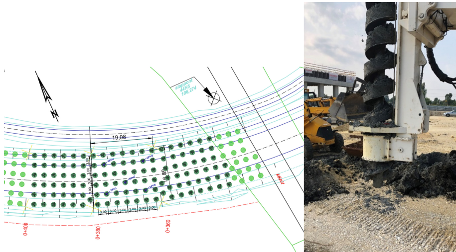
Fig. 19. Impulse Compaction ground improvement plan for a bridge ramp (left) and augering for gravel pillars (right)
