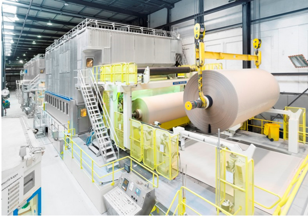
Fig. 1. A paper machine with jumbo rolls in the foreground (from VOITH)
