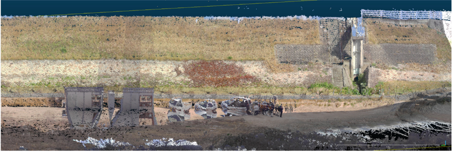
Fig. 6. Laser point cloud obtained by on-foot measurements on the inside of the levee using the portable laser measurement system
