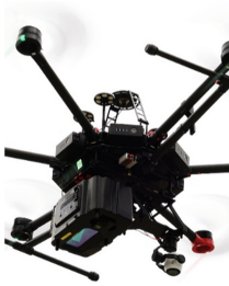
Fig. 1. Drone-mounted LiDAR system
