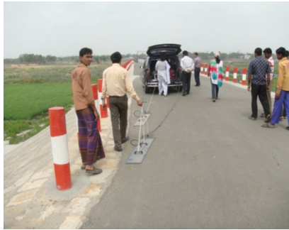
Fig. 2. Layout of GPR (1.2 m) test where a pair of 1.2 m antennas are used.
