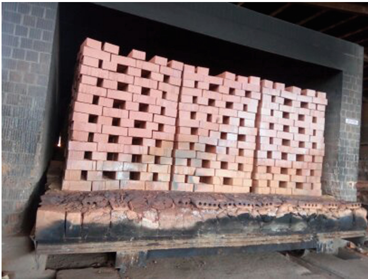
Fig. 3. Clay bricks after firing from the furnace
