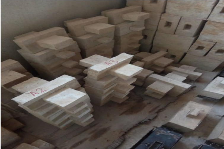
Fig. 2. Freshly demolded clay brick components
