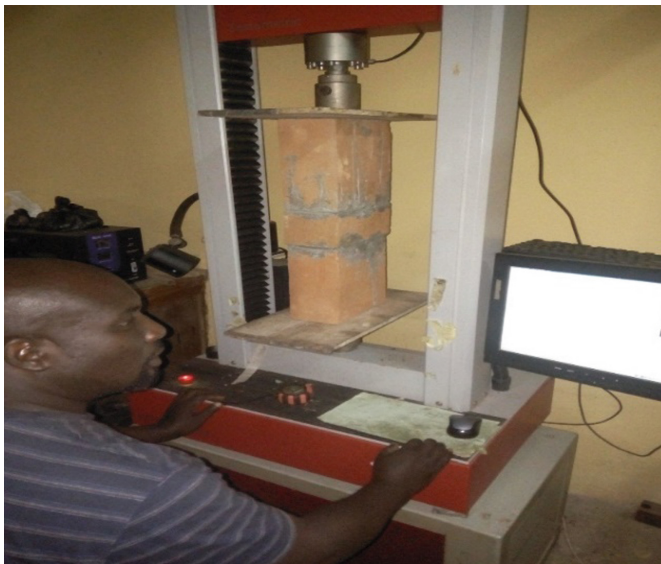
Fig. 5. Compressive test on clay brick
