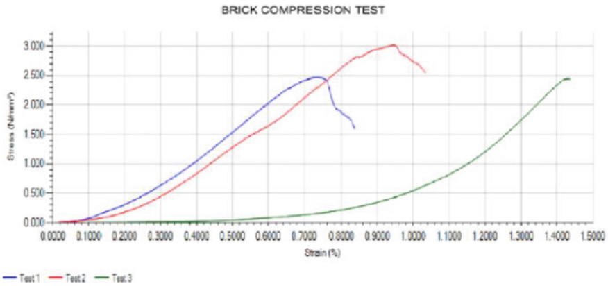
Fig. 8. Result of compression test for category A clay bricks
