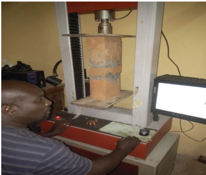
Fig. 5. Compressive test on clay brick
