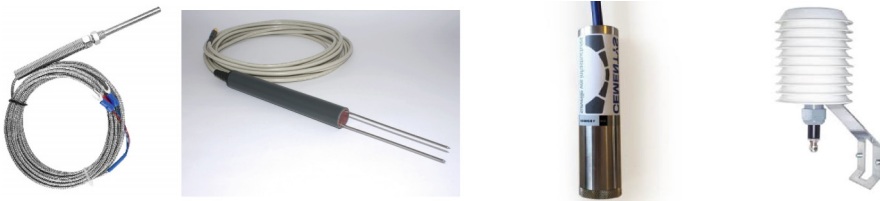
Fig. 5. PT100 sensors, TDR sensors, Vibrating wire sensors and Meteorological sensors (left to right)
