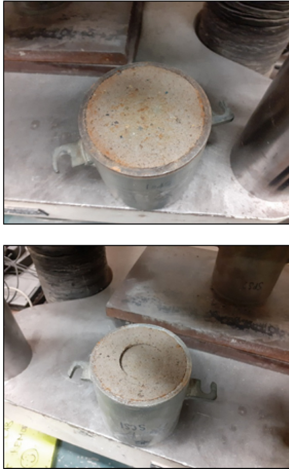
Fig. 4. Soil specimens before and after CBR test
