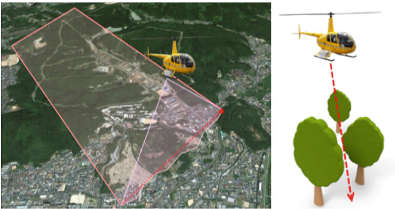
Fig. 1. Imaging diagram of aeronautical laser measurement
