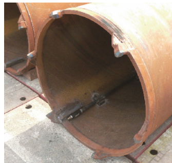
(b) Cutting bits and water pipe of rotary press-in pile
