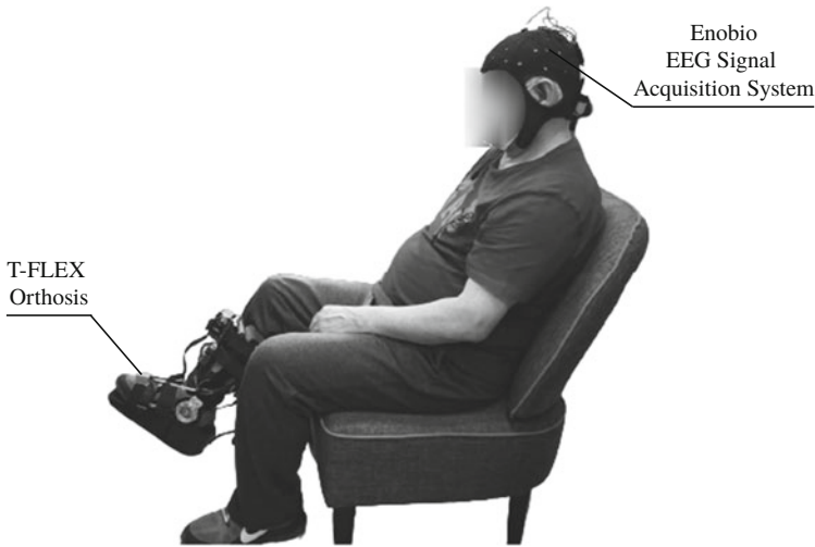
Fig. 9.3 Setup for BCI system integration with T-FLEX
