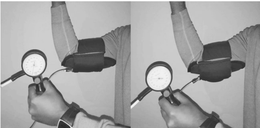
Fig. 3.13 An inflatable interface to adapt to multiple users and to set an exact strapping pressure
