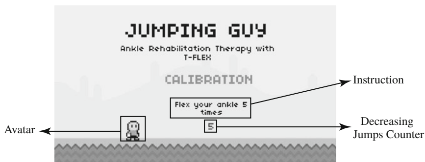
Fig. 12.8 Calibration interface. Request the execution of 5 movements of plantar and dorsal flexion. When the system detects a movement, the avatar jumps, and the counter decreases
