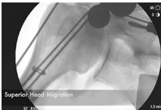
Fig. 3.7 Created irreparable posterosuperior defect leading to superior head migration and decreased acromiohumeral distance during abduction on a dynamic shoulder simulator
