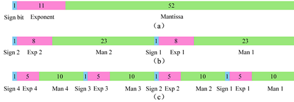
Fig. 4. Different precision floating-point formats used in the unit. (a) Double-precision format. (b) Single-precision format. (c) Half-precision format.
