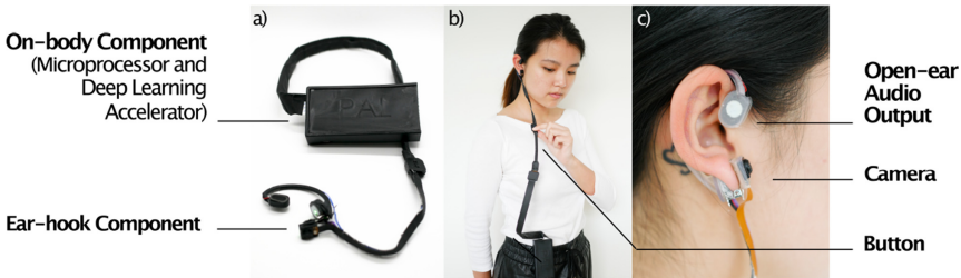
Fig. 3. (a) PAL’s full wearable device with an on-device deep learning accelerator, (b) worn by a person, (c) with a close-up of the on-ear camera and audio output.
