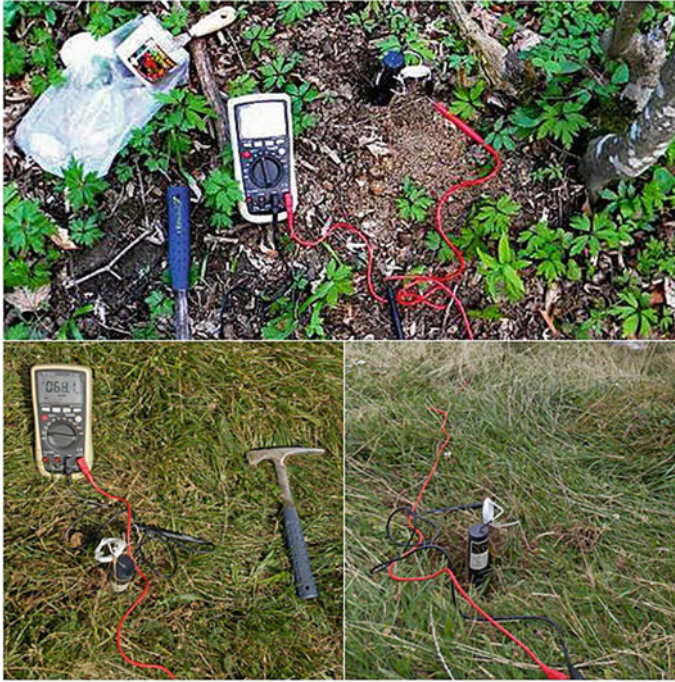
Fig. 9.4 Self-potential data acquisition in the field using a digital multimeter and the fix and mobile electrodes
