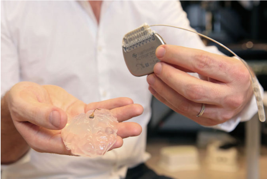
Fig. 3 The critical components of the brain-spine interface. Right hand: a 96-channel microelectrode Blackrock array is implanted into the phantom of the brain in the area corresponding to the leg motor cortex. These arrays are used to record action potentials of cortical neurons that represent movement attempts. The brain-spine interface acquires these brain signals to infer leg movement attempts. Left hand: a Medtronic implantable pulse generator connects to a multielectrode lead to form a spinal implant. Brain-spine interface uses inferred movement attempts to wirelessly control the spinal implant in real time. The spinal implant stimulates the spinal cord to reinforce the attempted movements, and therefore alleviate gait and balance deficits of Parkinson's disease
