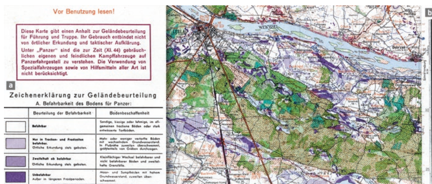
Fig. 12.13 Section of the legend (a) and map (b) of Panzerkarte: Sonderausgabe der Truppenkarte zur Geländebeurteilung (Panzer map: special issue of troop map for terrain evaluation) at the original scale of 1:100,000, sheet Piotrkow-Leslau-Sompolno-Klodawa, west of Warsaw, provided by the Forschungsstaffel in December 1944 (author’s collection)
