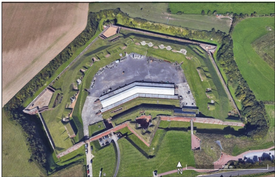
Fig. 3.14 Fort Nelson, Northern Approaches. Note the 'M'-shaped north caponier. (From Google Earth Pro; image Landsat/Copernicus 2020)
