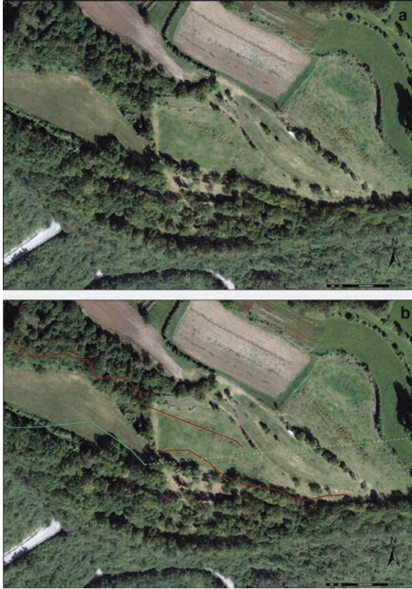
Fig. 6.6 (a) Orthophoto Reven flown in 2010. (b) The same air photo as (a) with trench traces identified by air photo interpretation (red). The dashed green line represents areas where no trench traces were identified during the ground survey, and the dark green line, areas where trench traces were still visible during the ground survey
