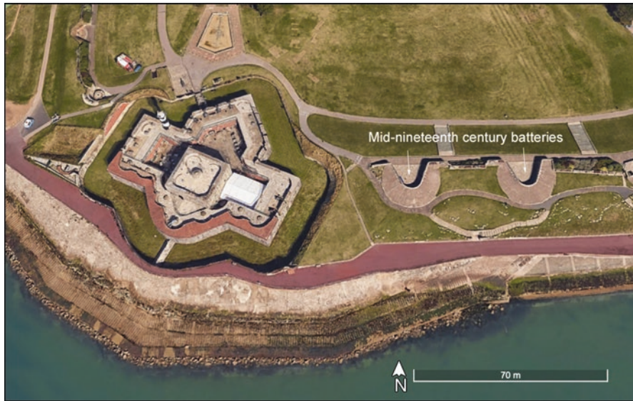
Fig. 3.8 Southsea Castle, a Phase 2 fort constructed in the trace-italienne style. The battery wings on either side of the Tudor fort were added in the mid-nineteenth century. (Modified from Google Earth Pro; image © 2020 Terrametrics)
