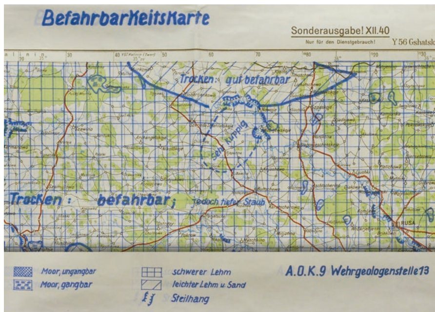
Fig. 12.7 Section of the 1:300,000 scale trafficability map, sheet Y56 Gshatsk (west of Moscow), provided by MGT13 of the Army High Command 9 in December 1940. Steilhang = steep slope, schwerer Lehm = heavy loam, ungangbar = impassable, Trocken: gut befahrbar = good going when dry. The map was printed as a special edition by the Reichsamt für Landesaufnahme (Reich Survey Office) in Berlin. (Used with permission from the Bundesarchiv/Militärarchiv in Freiburg im Breisgau, Document RH32/3098)
