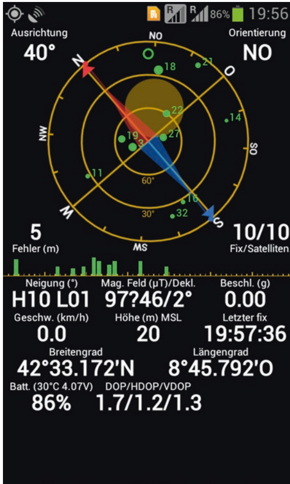
Fig. 18.5 Screenshot of a GNSS Android application, showing various satellite positions as well as the calculated coordinate solution (degrees North and East) with various parameters like geographic orientation, position calculation error, or signal strength
