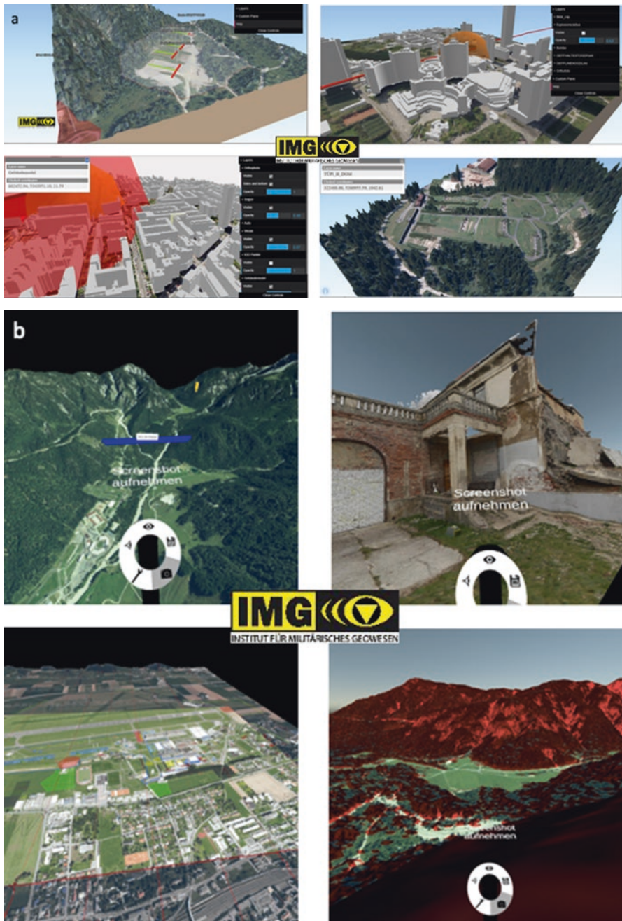
Fig. 18.3 Current developments in 3D geospatial models and virtual reality (VR). (a) Combination of screenshots from four different 3D models from tactical to urban warfare scenarios; the html format with limited GIS analysis functions (zoom, rotation, line of sight, or distance measuring) enables simple viewing (no additional software needed) in any standard browser. (b) Screenshots from within a virtual reality system: scenarios range from terrain to urban setting to buildings; the VR-controller can be seen at the bottom of the images and various active graphical inserts or analyses produced during the VR-session can be included; this tool is especially useful for terrain or geospatial evaluation and training
