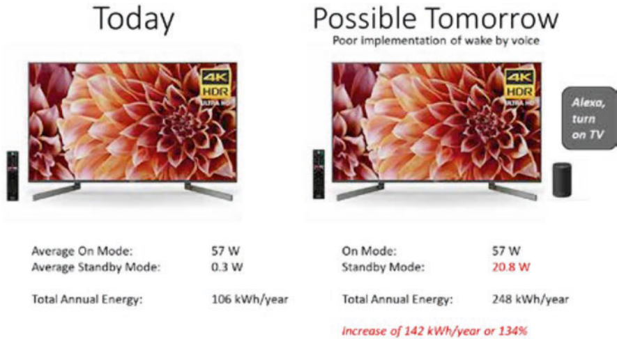
Fig. 1 Energy impact of wake by voice feature in TVs linked to a smart speaker
