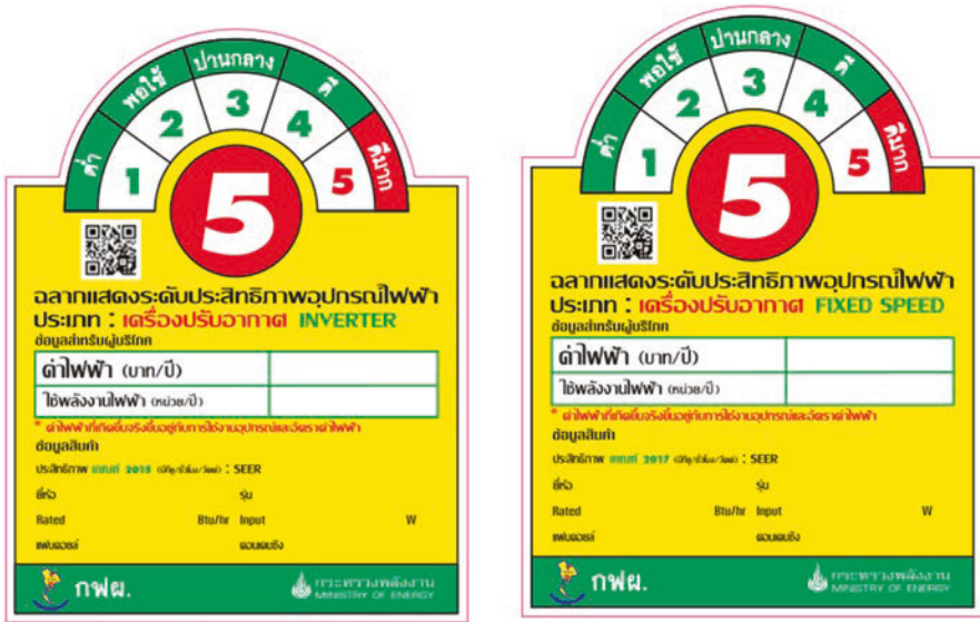
Fig. 7 2018 EGAT No. 5 labels for inverter (left) and fixed speed (right) ACs
