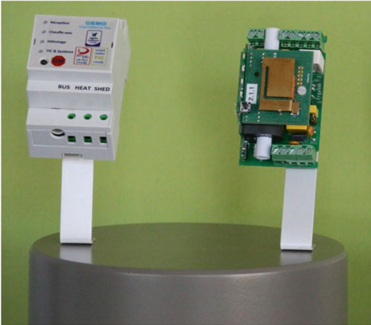
Fig. 2 The “GEMO”, the ultimate smart load controller (research prototype) (DEGETEL)
