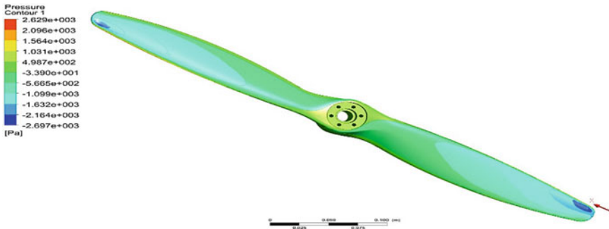
Fig. 19 Aerodynamic pressure distribution on the UAV’s propeller
