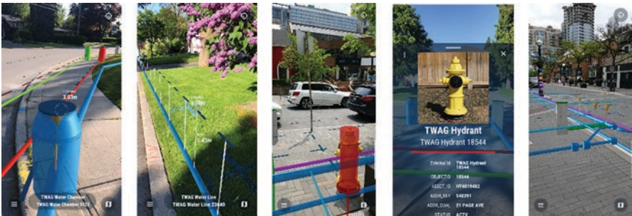
Fig. 9.9 Screenshots from the vGIS application showing AR scenes with additional annotations such as distances measured. (© vGIS Inc. All rights reserved)
