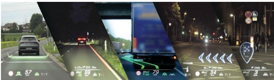
Fig. 9.4 Different AR features (left to right): Distronic (adaptive cruise control), lane departure warning, assisted lane change, route guidance, destination. (©Daimler Protics GmbH. All rights reserved)
