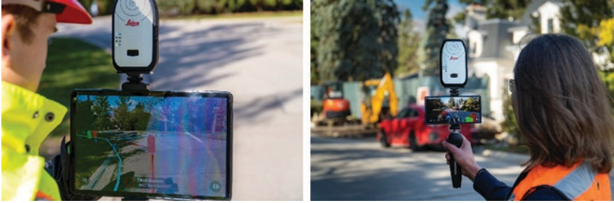
Fig. 9.8 Using smart devices with a location sensor to visualize underground infrastructure such as buried pipes and cables for construction: (a) with a tablet and (b) with a smart phone. (© vGIS Inc. All rights reserved)
