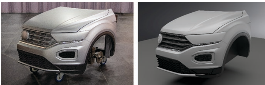
Fig. 9.1 A physical mock-up serving as a real model of the front part of a car in reality (left) and a virtual counterpart (right). (©Volkswagen AG. All rights reserved)
