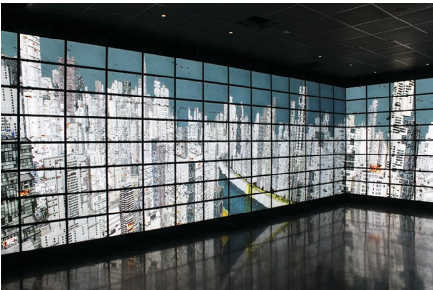
Fig. 5.34 Tiled wall of monitors illustrated by the Reality Deck at Stony Brook University
