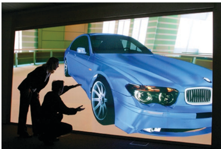
Fig. 5.32 Tiled wall using the example of the HEyeWall with 48 projectors. (© Fraunhofer IGD 2013, all rights reserved)
