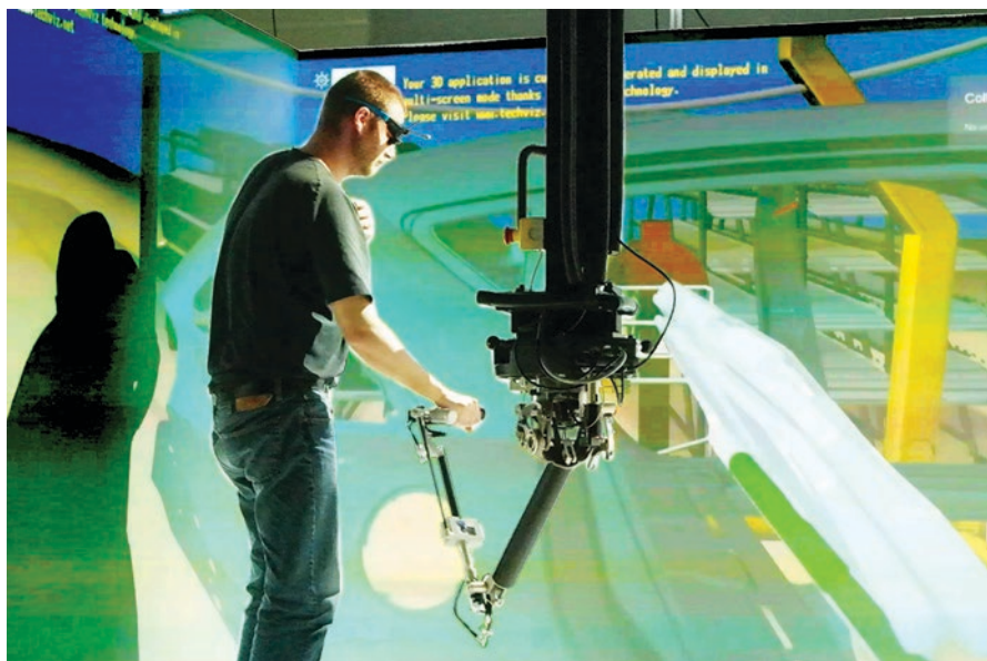
Fig. 5.47 Example of an end effector display. (© Haption SA, 2020. All rights reserved)
