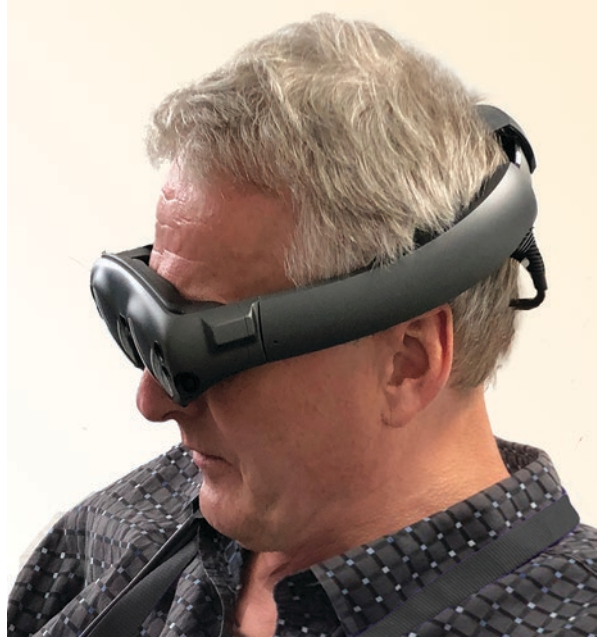
Fig. 5.23 Optical see-through AR glasses with integrated eye tracking (© W. Broll, all rights reserved)
