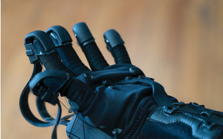
Fig. 5.45 Glove with pneumatic finger actuators and external skeletal structure. (© HaptX Inc. 2021. All rights reserved)
