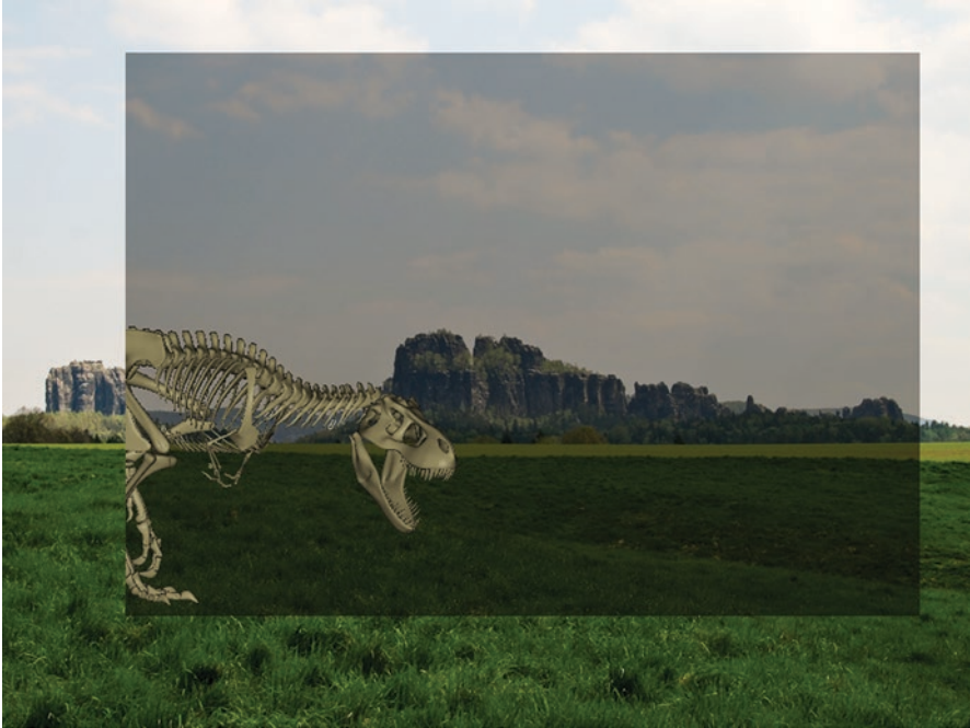
Fig. 5.21 Problems with the display of virtual objects at the boundaries of the field of view with an open design
