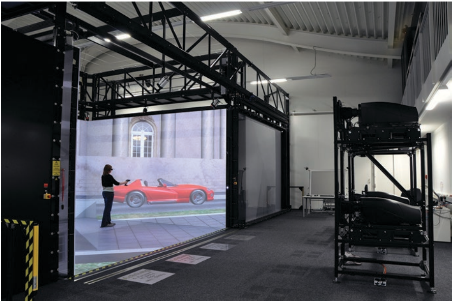
Fig. 5.2 CAVE-like multi-sided projection to visualize a design study (© RWTH Aachen 2013, all rights reserved)
