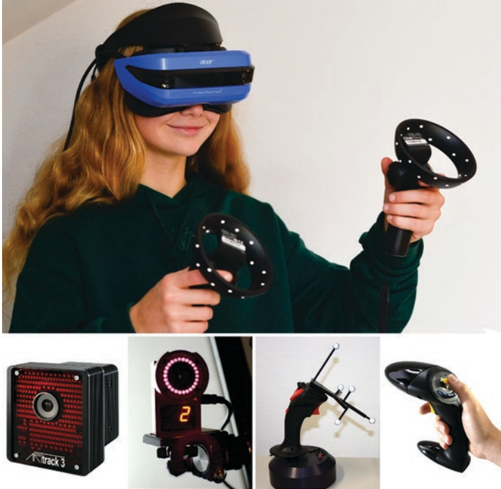
Fig. 4.4 (Top) VR controller with active marker; (bottom) cameras with infrared LEDs for illumination and flysticks with reflective markers
