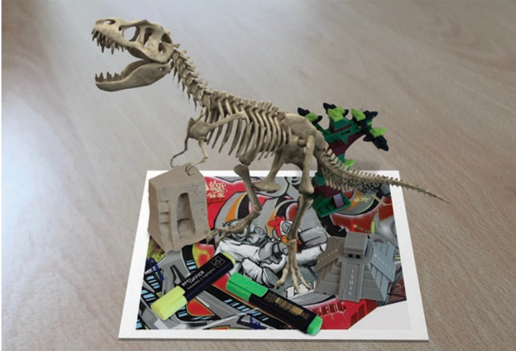
Fig. 4.13 Tracking based on features is much more robust against interference than marker-based tracking: despite numerous objects obscuring the image used for tracking, the virtual object can be registered correctly
