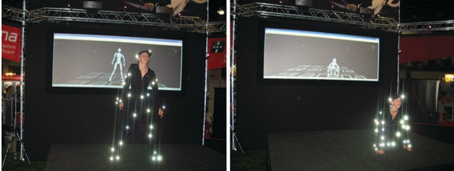
Fig. 4.7 Optical tracking of a person with reflective markers (the markers appear to be illuminated by the flashlight used) and several infrared cameras (infrared LEDs appear red)
