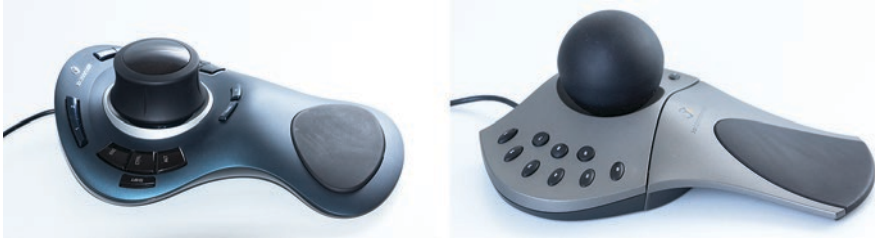
Fig. 4.24 Different variants of a 3D mouse
