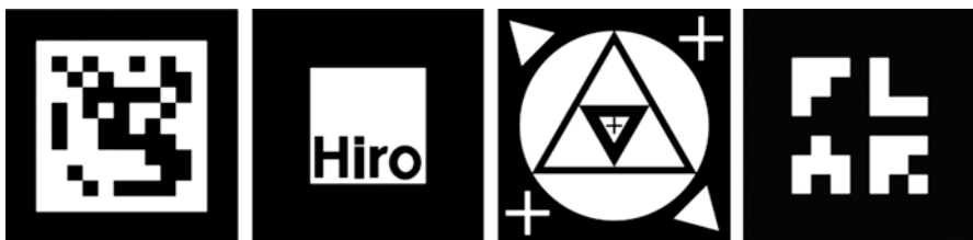
Fig. 4.8 Typical markers as used for camera-based tracking
