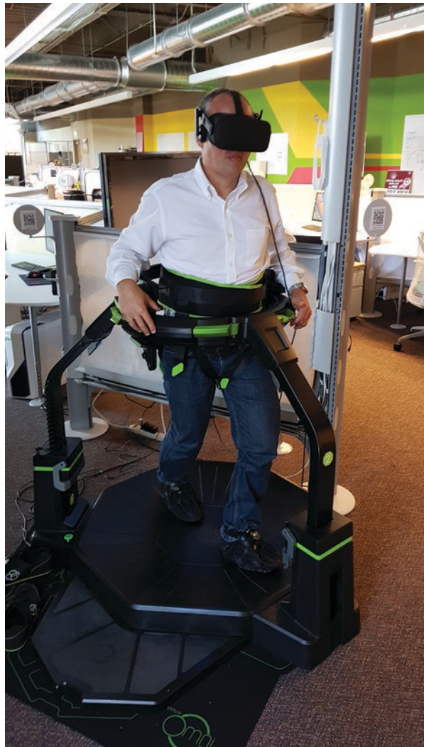
Fig. 4.26 User with VR glasses on an omnidirectional treadmill
