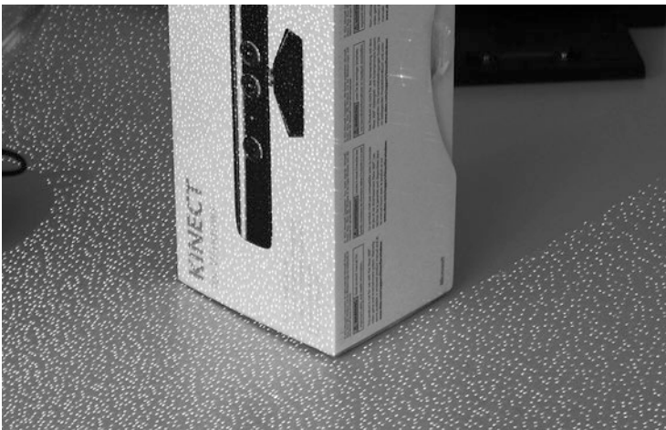
Fig. 4.14 Projected infrared pattern for depth detection of an RGBD camera. (© DLR 2013, all rights reserved)
