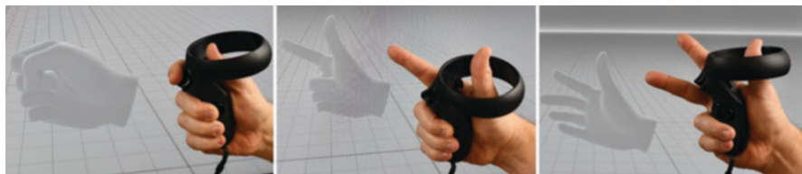
Fig. 4.18 3D model of a hand controlled by a VR controller with touch sensors
