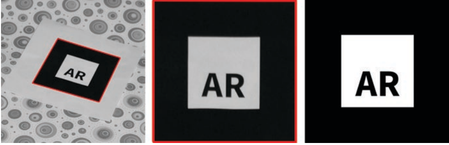
Fig. 4.10 Recognized marker, normalized marker, normalized original
