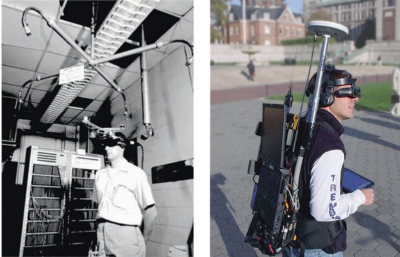
Fig. 1.7 Pioneering work in the field of VR/AR. (Left) Sutherland’s data glasses with 6-DOF ultrasound tracking; image courtesy of © Ivan Sutherland, all rights reserved. (Right) Replica of the MARS system of 1997 (Bell et al. 2002). (Image courtesy of © Steve Feiner, all rights reserved)
