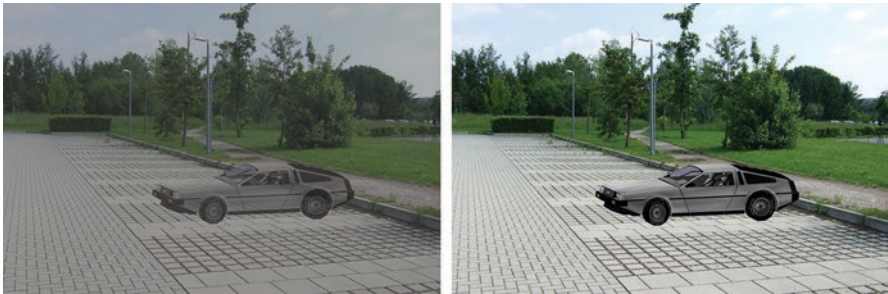
Fig. 8.9 Typical perception when using the optical see-through technique (left) compared to the video see-through technique (right)
