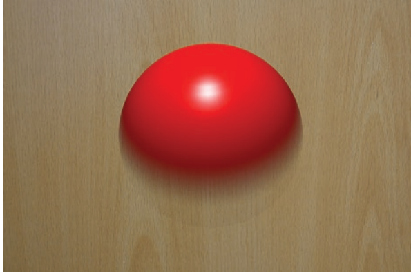
Fig. 8.8 With the OST AR techniques, dark virtual objects sometimes appear transparent (here the less illuminated lower part of the red sphere)
