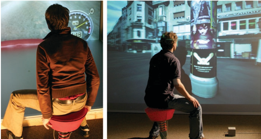
Fig. 6.5 The ChairIO allows navigation in a virtual environment by leaning in the desired direction of movement. To implement this concept, a special chair was equipped with additional sensors according to Beckhaus et al. (2007). (© Steffi Beckhaus. All rights reserved)
