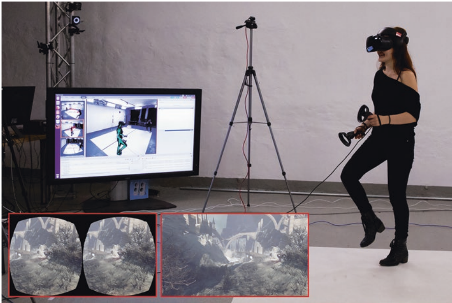
Fig. 6.4 The figure shows a simple “walking in place” method where a user is tracked by a mobile motion capturing system. The body movements are detected by inertial sensors at the joints and control movement and orientation in the virtual environment. On the bottom left, the user’s pre-distorted view (see Chap. 5), which is generated for both eyes, is shown. (© Christian Geiger, HS Düsseldorf. All rights reserved)
