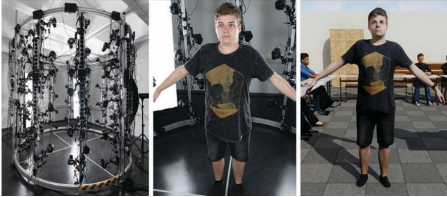
Fig. 9.22 Photogrammetry system at the Chair of HCI at the University of Würzburg with about 100 SLR cameras for photorealistic 3D reconstruction of user avatars. Left: The multi-camera system that was initially used. Center: A user during the 3D scan process. Right: The result of the reconstructed avatar in a virtual scene. Figure adapted from Latoschik et al. (2019). (© ME Latoschik et al. All rights reserved)
