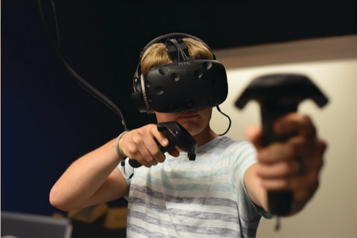
Fig. 5.1 Typical consumer HMD with integrated head-tracking and accompanying controllers (© TU Ilmenau 2019, all rights reserved)
