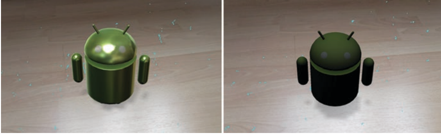
Fig. 10.9 Illustration of the illumination in ARCore with a 360° HDR ambient illumination in HDR (left) and simple intensity detection (right). Metallic objects in particular benefit from the 360° illumination reconstruction
