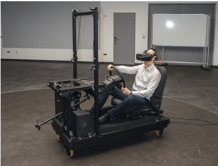
Fig. 9.2 A seating buck as shown in this picture is used to provide haptic feedback for an immersive experience in VR. (©Volkswagen AG. All rights reserved)
