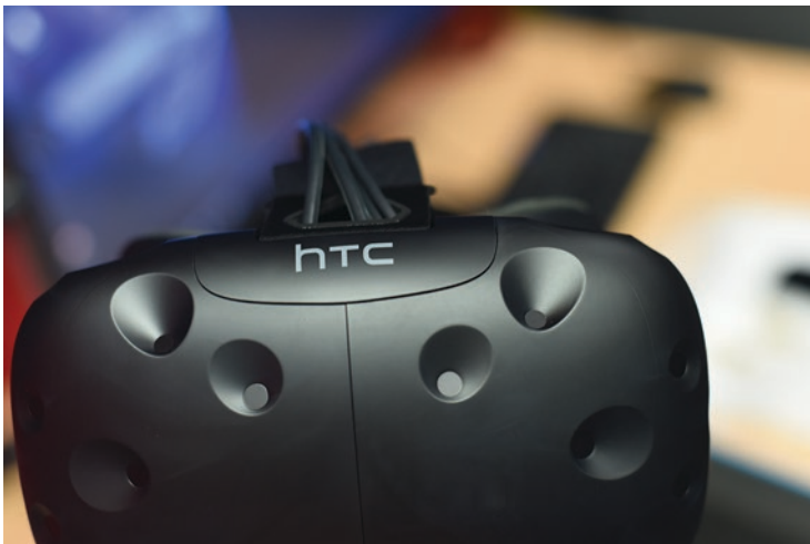
Fig. 5.6 Typical representative of consumer VR glasses with integrated sensors for tracking (© TU Ilmenau 2019, all rights reserved)
