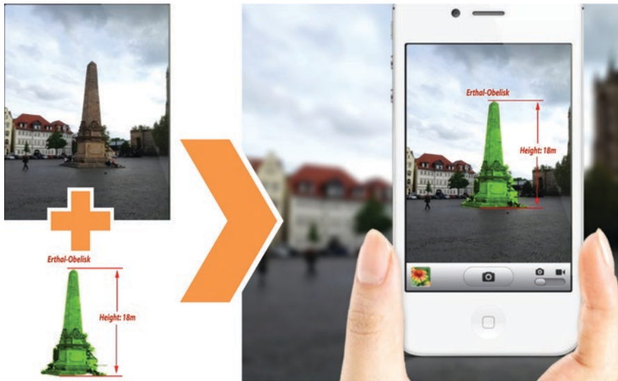
Fig. 8.6 Perspectively correct superimposition of a camera image of the real environment by virtual content using video see-through AR – here on a smartphone
