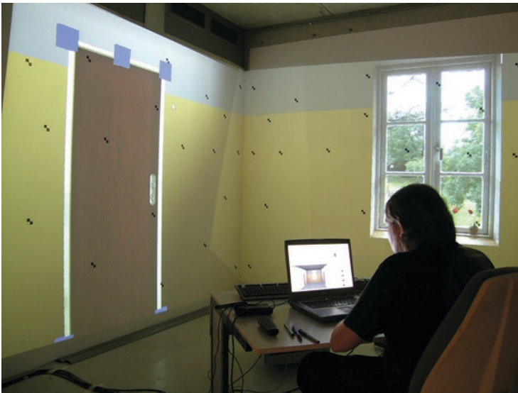
Fig. 8.7 Example of projection-based AR (virtual door, virtual color design of the wall). (© Oliver Bimber 2005. All rights reserved)
