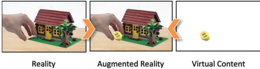
Fig. 8.1 Fusing a real environment (left) with a virtual object (right) to achieve Augmented Reality (center). (Single images: © Tobias Schwandt, TU Ilmenau 2018. All rights reserved)
