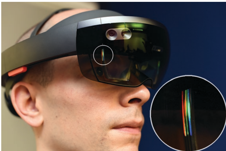
Fig. 5.10 HMD with clearly visible waveguides for the individual color channels (see magnification) (© TU Ilmenau 2019, all rights reserved)
