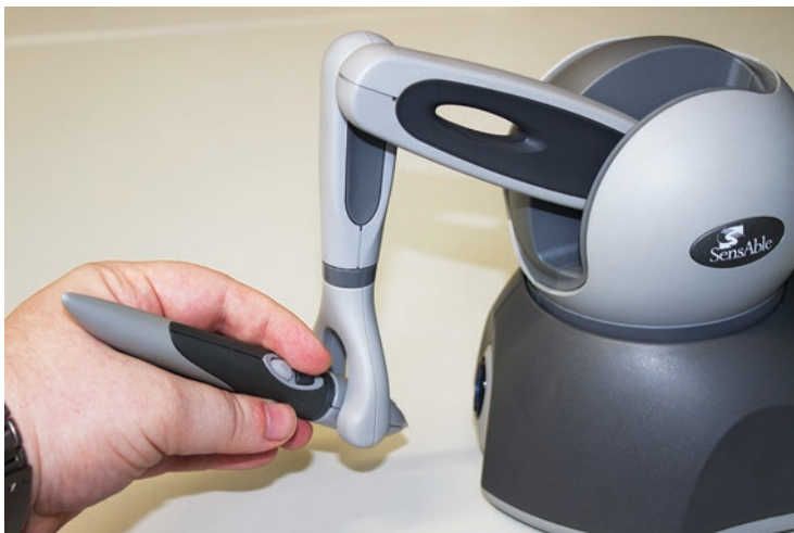
Fig. 4.25 Mechanical input device in pen form with haptic feedback
