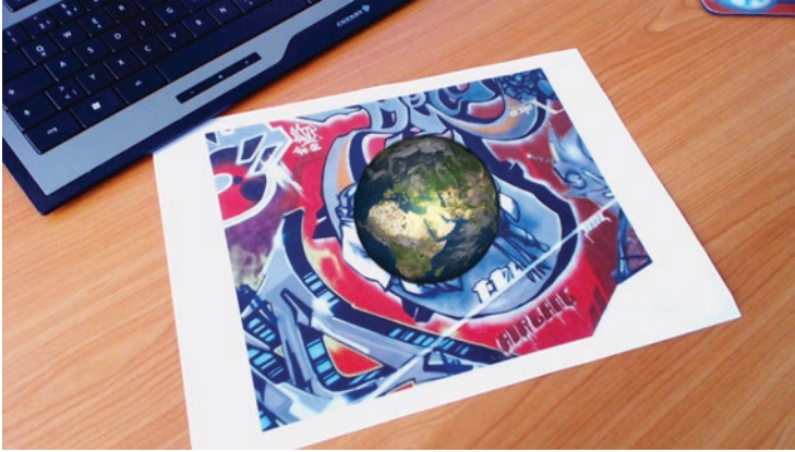
Fig. 8.3 Perspective superimposition of an image used for tracking by a 3D object. (Image source: Jan Herling, TU Ilmenau)
