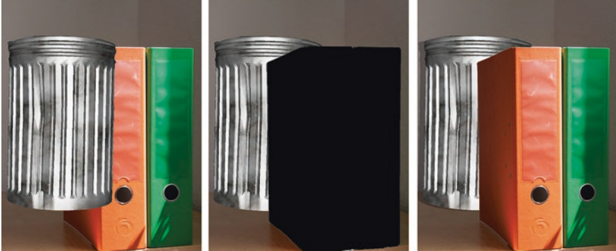
Fig. 8.22 Phantom objects enable correct mutual occlusion between real and virtual objects. Without a phantom object, the virtual object seems to float in front of the real objects, whereas with correct masking by the phantom object it seems to be behind the real objects
