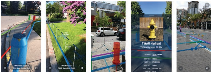
Fig. 9.9 Screenshots from the vGIS application showing AR scenes with additional annotations such as distances measured. (© vGIS Inc. All rights reserved)
