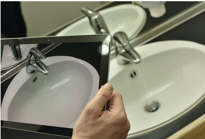
Fig. 8.27 Example of diminished reality: the sink drain is removed from the live video stream in real time. (© TU Ilmenau 2018. All rights reserved)
