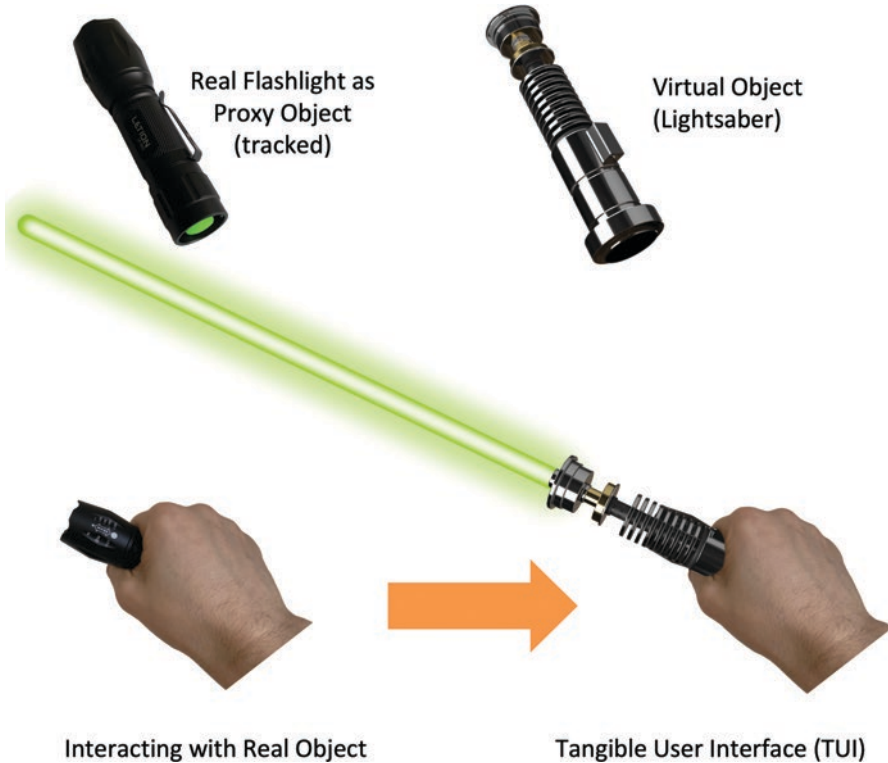
Fig. 8.26 Tangible User Interfaces: a real proxy object is used to interact with a virtual object
