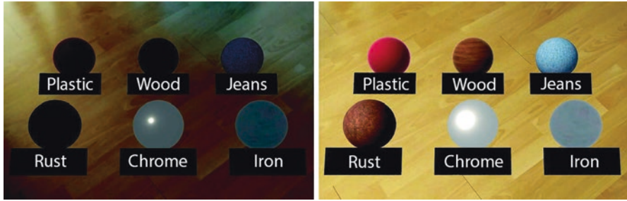
Fig. 10.20 Illustration of two differently illuminated scenes and the influence of the illumination situation on the material properties
