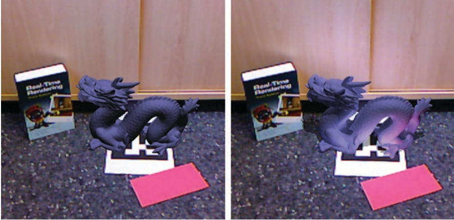
Fig. 8.15 Comparison of an AR scene without and with photometric registration: in the right image, (real) light is reflected by the red sheet onto the virtual object; furthermore, light from the virtual object is reflected onto the background. (Picture source: Philipp Lensing, TU Ilmenau)
