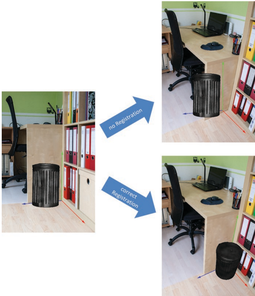
Fig. 8.10 Left image: Correct geometric registration of the virtual trash can. Image top right: Virtual object is displayed at the same position as in the left image, but it is geometrically not registered with the surrounding reality. Image bottom right: Based on the tracking data, the correct perspective of the virtual object is displayed from the current viewpoint and the current viewing direction of the camera; the virtual object is geometrically correctly registered with the surrounding reality
