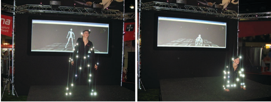
Fig. 4.7 Optical tracking of a person with reflective markers (the markers appear to be illuminated by the flashlight used) and several infrared cameras (infrared LEDs appear red)
