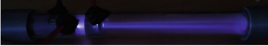
Fig. 7 Successful electron beam generation in the 3D-printed plasma cathode electron gun
