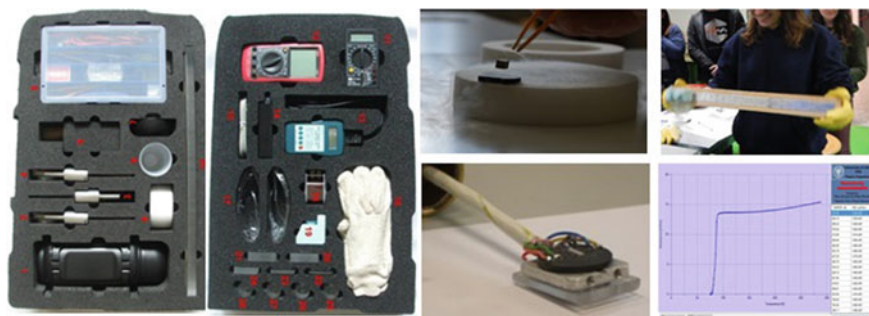
Fig. 1 High tech kit for exploring superconductivity (left) and examples of experiments (right, from the top): Meissner effect levitation of a magnet on a superconductor; model of MAGLEV train; apparatus for measurement of the breakdown of resistivity in superconductors and sample data
