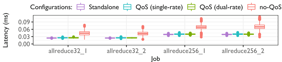
Fig. 4. Distribution of MPI_AllReduce operation latency across the ranks of each allreduce jobs. We achieve near baseline (Standalone) latencies when allreduce jobs use the low latency class of the dual-rate and single-rate QoS configurations.
