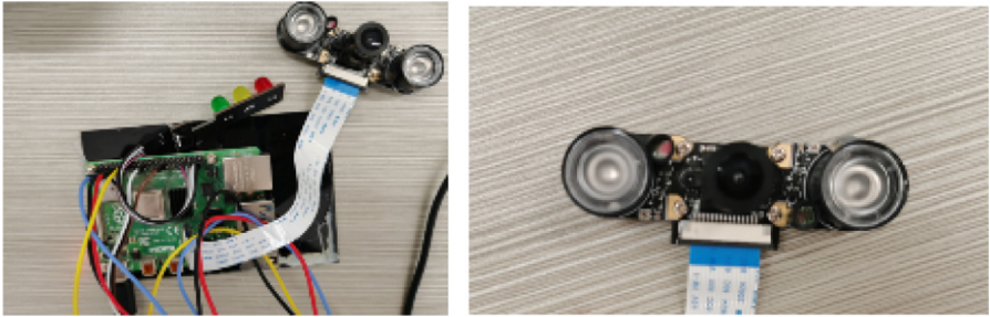
Fig. 6. The overall situation of the equipment. The infrared camera is connected to the Raspberry Pi 4 Model B through the CSI interface. In order to be able to prompt alarm data, the Raspberry Pi is connected with a micro display, LED lights.
