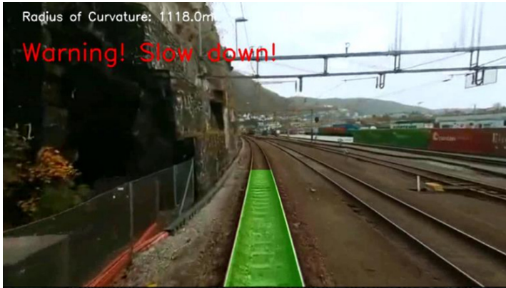
Fig. 4. The curved track early warning
