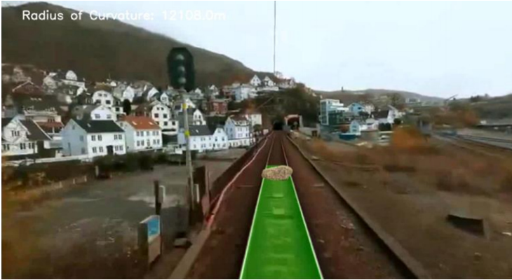
Fig. 6. The obstacle detection early warning
