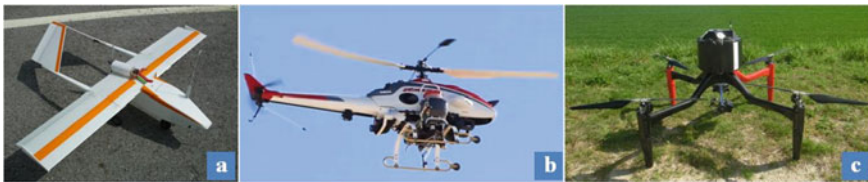
Fig. 4 Three examples of UAVs: a fixed-wing; b helicopter; c quadrotor (after Valavanis et al. [45], SpringerLink)
