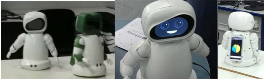
Fig. 1. The STIMEY Robot Prototype, left: two different versions of the robot, middle: happy facial expression, right: the robot's back with the embedded mobile phone device.
